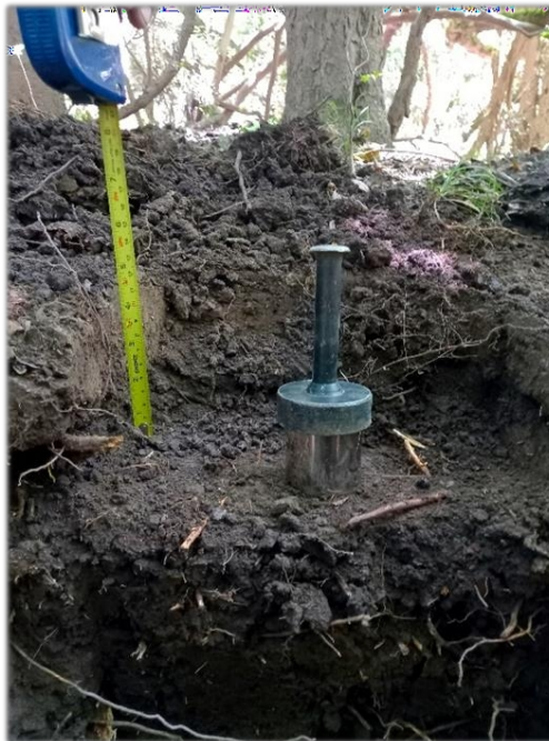
Figure 31: Collection of undeformed soil samples using the volumetric ring method.
