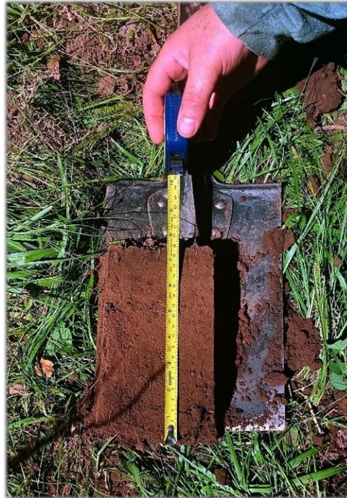
Figure 30: Soil sampled at various depths for analysis of total carbon content in the laboratory.
