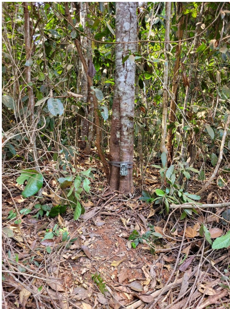
Image 3.1-66: Camera-trap installed in the project area (Author records, August-2023).
