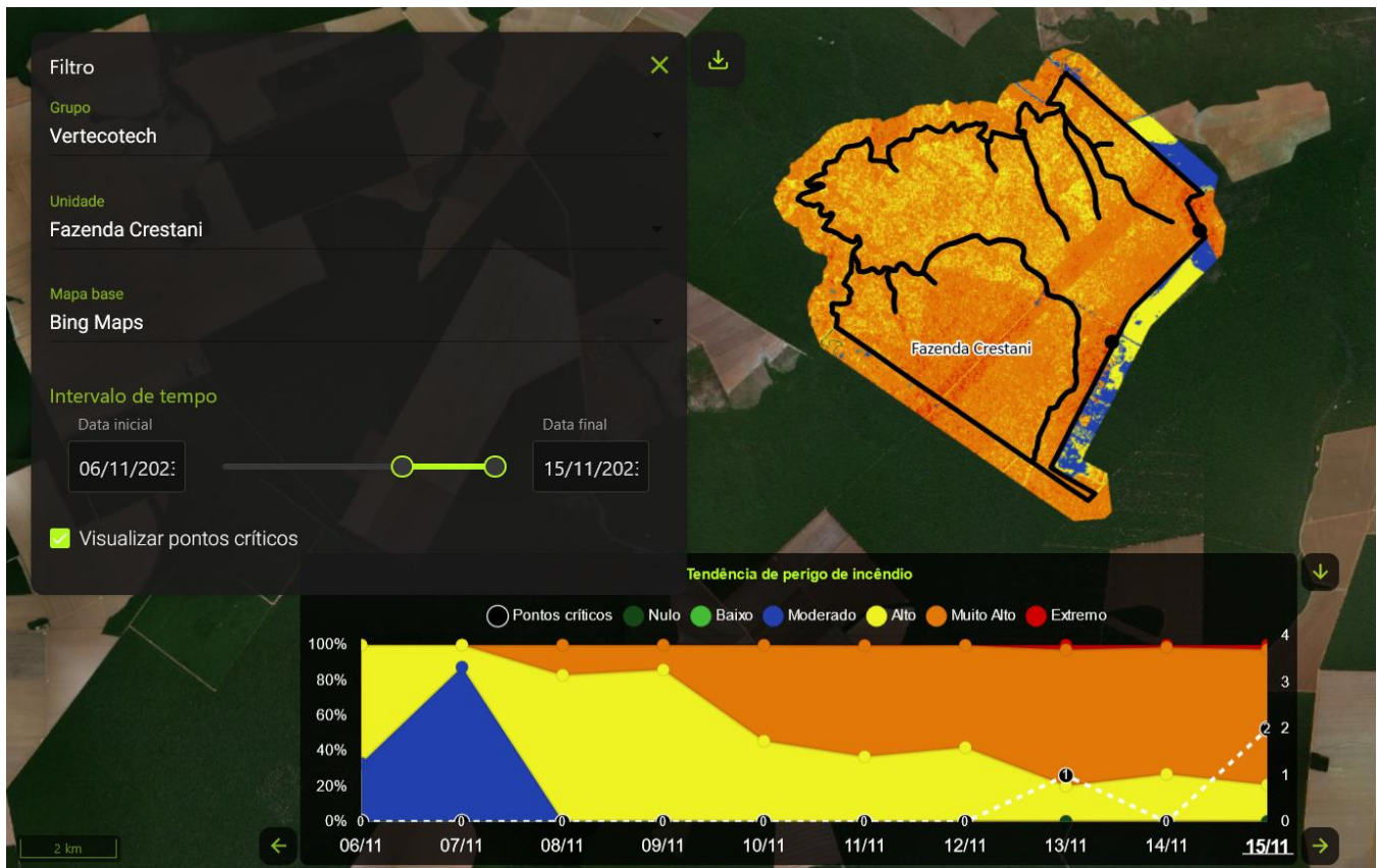
Image 3.1-11: Quiron’s monitoring platform in Vert Ecotech’s module, with 3 critical points suggested in “very high” (Muito Alto) for fire risk in the buffer perimeter (500 m) – from 06 to 15 of November-2023.
